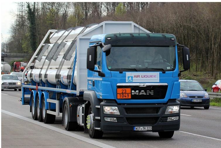
Figure 3 Typical gaseous tube trailer [Air Liquide]
